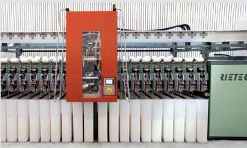
Fig. 2 The new J 10 air-jet spinning machine with four robots
