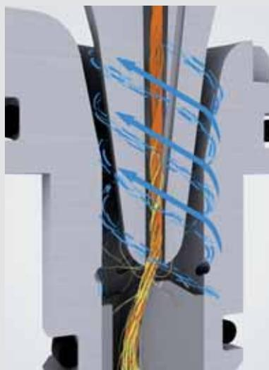
Fig. 6 Diagram of the ComforJet® piecing in the spinning nozzle (yarn – orange; new fibers – yellow; air current – blue)
