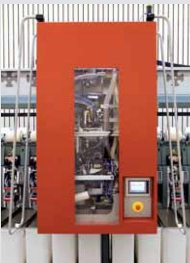
Fig. 5 Invisible piecing by the robot on the J 10
